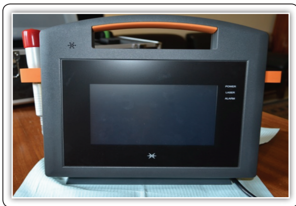
FIG (2a) Gallium Aluminum Arsenide semiconductor diode laser equipment used in the study.
