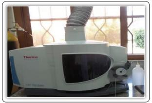
FIG (3) Ion chromatography instrument.
