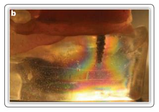
FIG (1) (a&b): Fringes order around dental implant with nylon framework under stress
