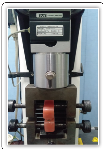
FIG (2) Universal testing machine used the retentive force for each prosthetic component at a crosshead speed of 50 mm/min.
