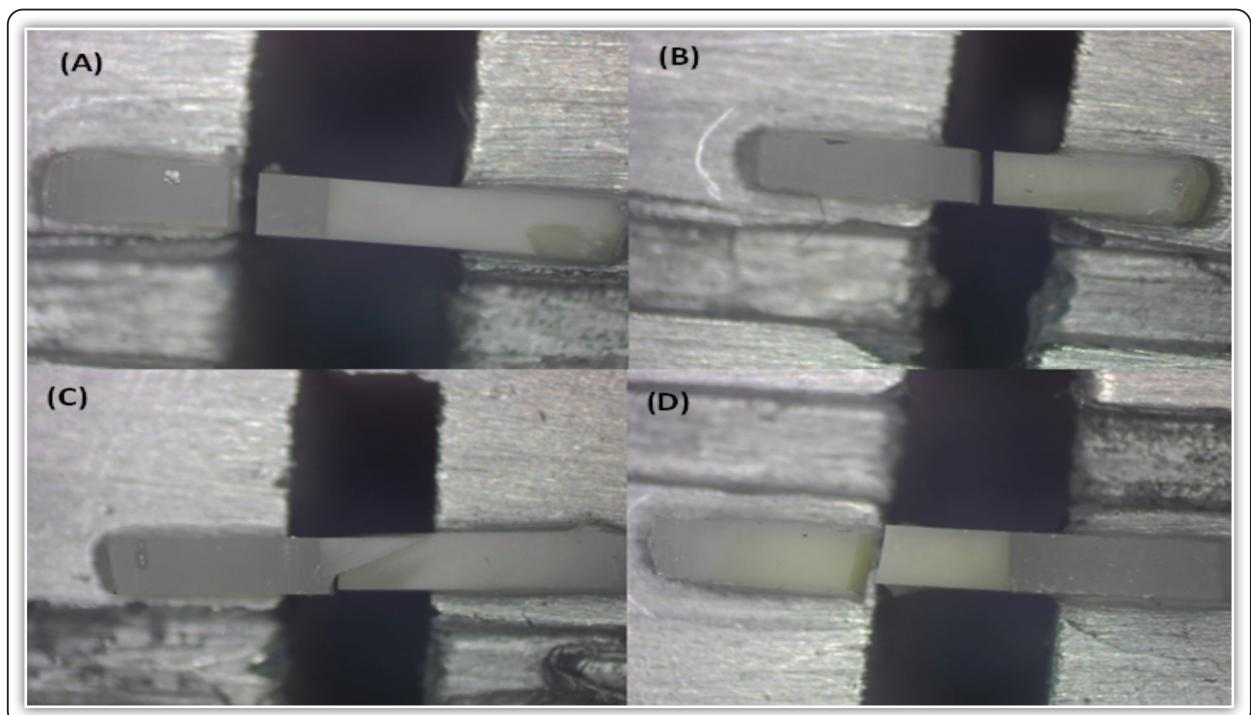
FIG (3) Showing stereomicroscopy image (A) showing cohesive composite failure (B) showing adhesive bond failure (C) showing mixed cohesive adhesive failure (D) showing cohesive dentin failure
