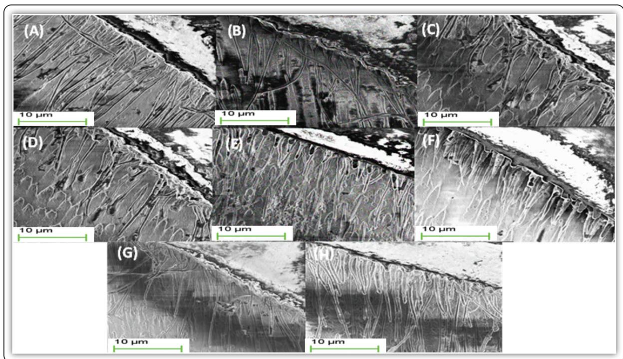
FIG (1) Showing SEM images showing (A, C, E, G) resin tags in control, minocycline, chlorhexidine and sodium hypochlorite groups respectively before thermocycling and (B, D, F, H) resin tags in control, minocycline, chlorhexidine and sodium hypochlorite groups respectively after thermocycling.
