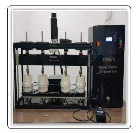
FIG (2) Each clasp and its models were mounted on the chewing simulator device.
