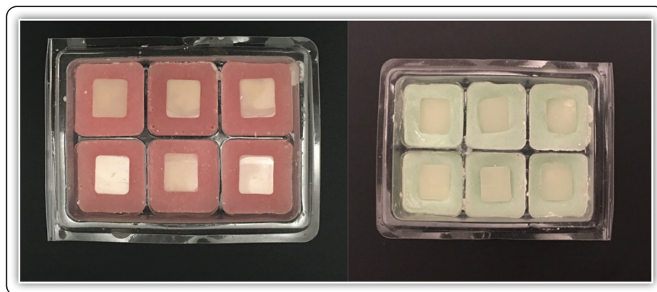
FIG (1) Acrylic blocks with embedded CAD/CAM discs
