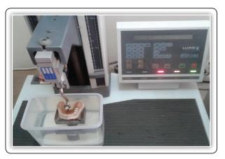
Fig. (1) Retentive force evaluation using the Universal testing machine.
