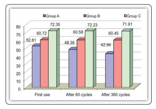
Fig. (2) Tensile load (in Newton) required to remove the RPD from the acrylic cast at the first time of use, after 60 cycles and after 360 cycles of insertion and removal for Co-Cr, flexible and AuNps reinforced flexible RPDs.
