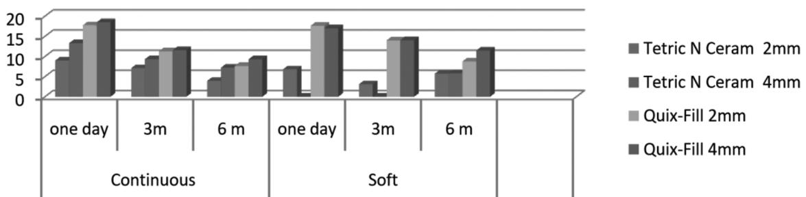
ed statistically significant ( $p < 0.05$ ) highest shear bond strength mean values (13.625), followed by 3 months storage time group mean values (10.067), while the lowest statistically significant ( $p < 0.05$ ) shear bond strength mean values recorded after 6 months storage time group (7.48).
