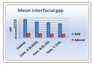
Fig. [2]: Column chart showing mean marginal gap (µm) in both sealers with different NAgPs concentrations.
